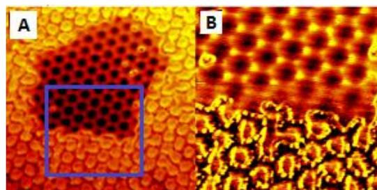
Figure 3 Desorption of hydrogen on graphene on Ir(111) A) 300Åx300Å, -449mV, -0.490nA B) 150Åx150Å, -449mV, -0.470nA, a high resolution image of the area marked with blue in A).
