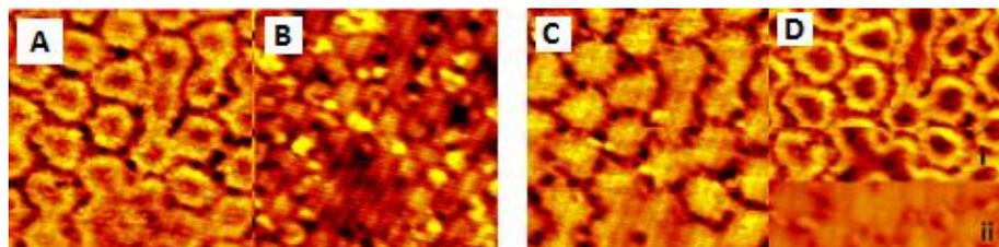
Figure 2 Full coverage of hydrogen on graphene on Ir(111) 100Åx100Å A) +657.2mV, +0.370nA B) +1314.4mV, +0.370nA C) -657mV, -0.370nA, D) 100Åx100Å i: -423mV, -0.360nA ii: -1314.4mV, -0.350nA
