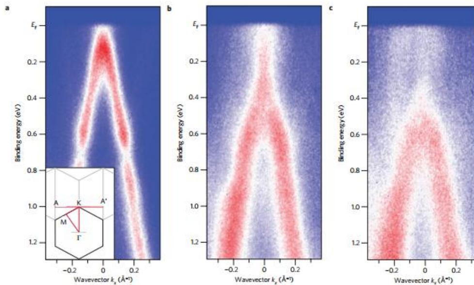
Figure 1  $\pi$ -band images of graphene obtained by ARPES a) clean graphene on Ir(111) b) graphene on Ir(111) exposed to 30s dose of atomic hydrogen c) graphene on Ir(111) exposed to 50 s dose of atomic hydrogen [3].
